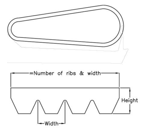
$\begin{array}{ll} \text{Datum Llength} = 2337 \\ \text{Height} &= 3.5 \\ \text{Number of ribs} = 8 \\ \text{Pitch} &= 2.34 \\ \end{array}$
